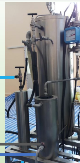
CO 2 storage tank
